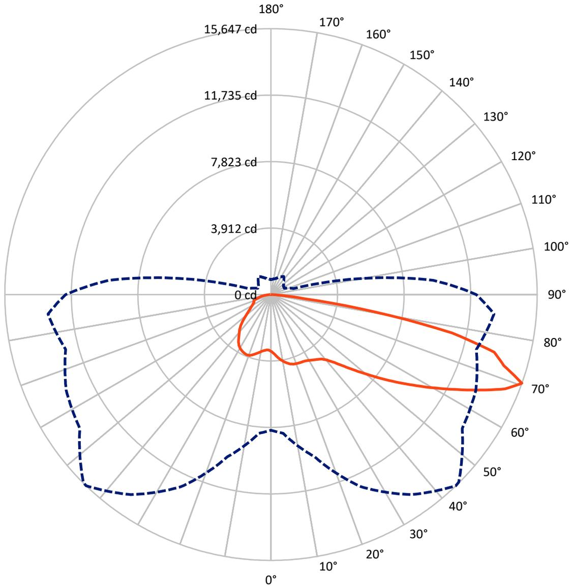
— Vertical Plane Through 44-Deg Lateral    - - - Horizontal Cone Through 70-Deg Vertical
