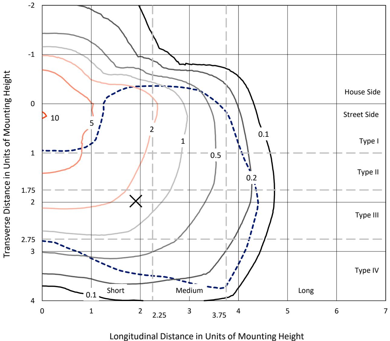
Based on 20 foot mounting height. Maximum calculated value = 10.3 fc
